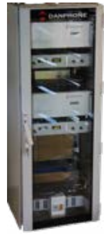
NAVTEX rack with two redundant transmitters
