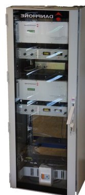
NAVTEX rack with two redundant transmitters
