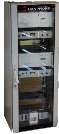
NAVTEX rack with two redundant transmitters
